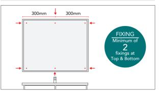
Securely fasten cabinet to the wall through back with appropriate screws/bolts at TOP and BOTTOM of cabinet. Evenly space apart the horizontal fixings at a maximum of 300mm apart.
