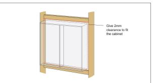
Complete Step 1, cut a hole 4mm bigger than the overall cabinet carcass in the wall. Position and secure cabinet in cut out, go to Step 2.
