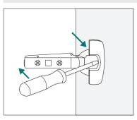
Once you have removed door from the cabinet, using a flat head screw driver, lift and release the top cover plate.
