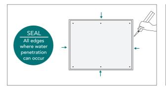
Apply non-acidic silicone to all edges where cabinet meets the wall. **Note:** Gap sealant can be used in place of silicone where the unit meets tiled surfaces.
