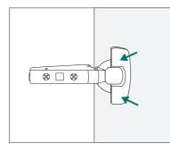
Once secured in position, click cover plate down to lock into place.
