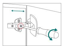
Use front screw to move door to the left or right, or to level each door.
