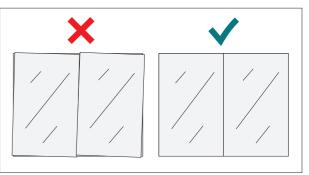
Install doors back onto cabinet and make adjusments to align the doors correctly. See opposite page for instructions.
