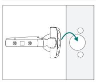
With top cover plate lifted, place hinge into position on door and insert into holes until flush.
