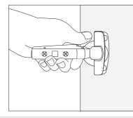
Pull hinge up and out from door. You may need to wiggle the hinge to loosen and use a little force.
